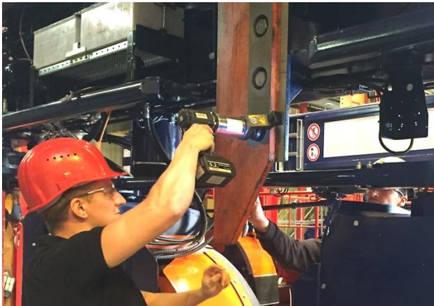
**Designed for service jobs:** These bolts of a ship container loader („straddle carrier”) are tightened quickly and precisely with an ITH ADS-150.
