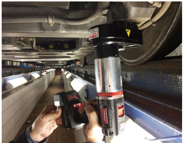
Picture 3: M20 bolt connections of a shock absorber on a railway vehicle are precisely tightened with an ITH ADS 75 Digital to 450 Nm (331 ft*lbs). An ITH Side-drive is used to provide an optimal reaction point.
