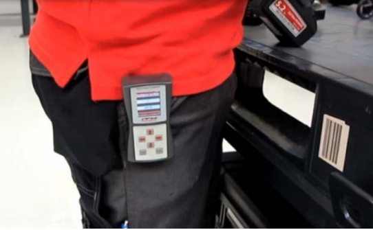
Picture 5: Patent-protected wireless control "ADS Smart Control" can be attached to the user's clothing with the robust clip mechanism. By separating electronics from the Nut Runner, the risk of damage to the electronics is nearly eliminated.
