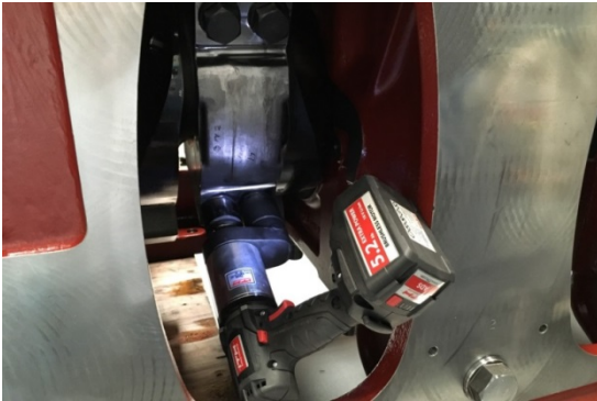
Picture 6: When torqued, high-load bolts are often tightened using the torque-angle method. The connecting rod bolts of a large diesel engine in this picture are subjected to high dynamic loads and are precisely tightened by an ITH Nut Runner type ADS.
