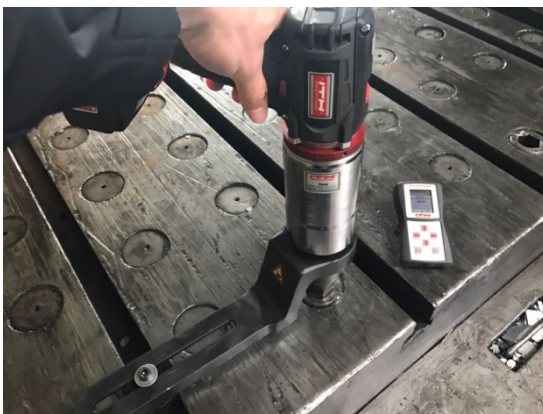
Picture 7: With a custom reaction arm, these M30 hexagon bolts are tightened by an ITH Battery Nut Runner type ADS Digital.
