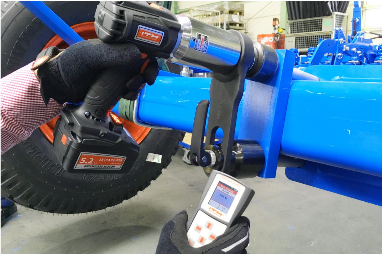
Picture 1: Wireless handheld digital control “ADS Smart Control” manages all relevant application data for one or more ITH Battery Nut Runners type ADS Digital. Pictured above, axle connection bolts of an agricultural machine are precisely tightened to 1.000 Nm (738 ft*lbs).
