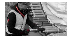
**Battery-Nut Runner Type ADS** Up to 6,000 Nm (4,440 ft\*lb), class-leading weight-to-power ratio, documentation.
